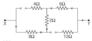
Equivalent resistance between X and Y  $R_{\rm eq}$  =  $8+2+6=16\Omega$
