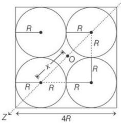
Moment of inertia of one hole at about Z-axis
